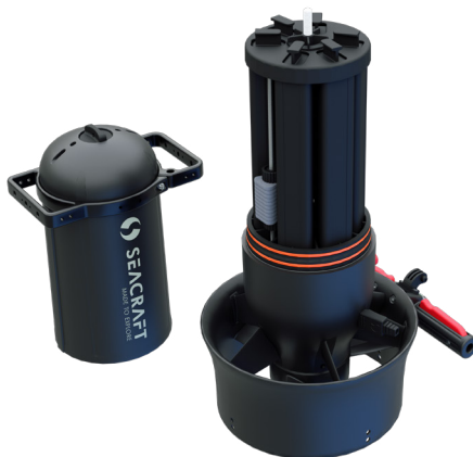
Figure 10. GO! Scooter after opening with visible ballast system
