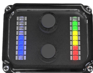
Figure 22. GO! scooter display – gear 4 selected, battery approximately 88%
