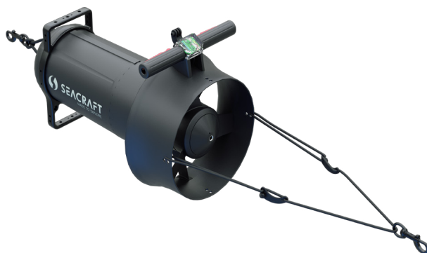
Figure 13. Scooter harness mounted on the scooter nozzle
