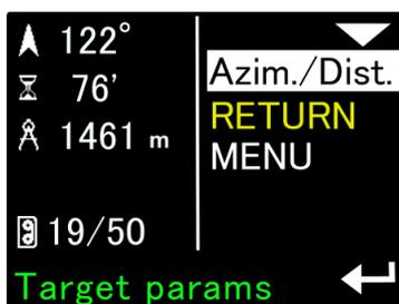
When we select the option Az./Dist. , the device will go to the screen that allows you to program the parameters of our target (azimuth and distance):
