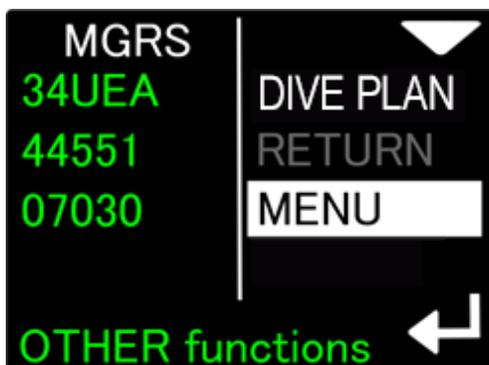
Currently, the current reading of GPS coordinates in the MGRS record is also displayed in the same place, alternating with the date / time and temperature (every 3 seconds change).
