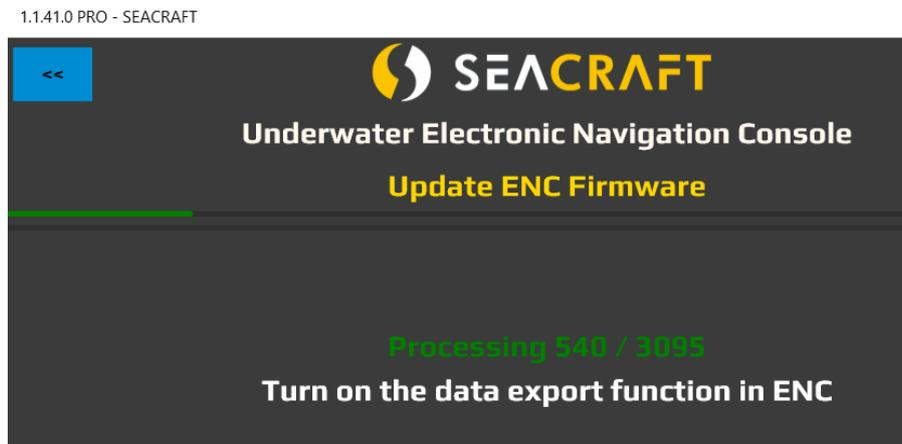
The progress bar and green text show the progress of the operation. When the data transfer is complete, the ENC console will restart automatically and start installing new software. This process may take about 1 minute.
