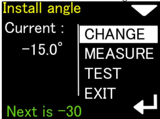
The lower button allows you to cyclically change the installation angle: - 20 / - 30 / - 40 and again -20 ...
