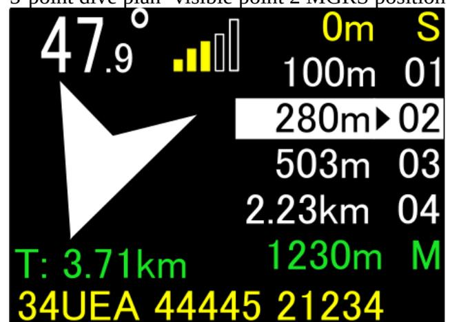
The bar indicator at the top of the screen shows the quality of the current GPS signal and can be green (Very good) or yellow (Fair). No GPS signal at the moment is indicated by empty bars.
