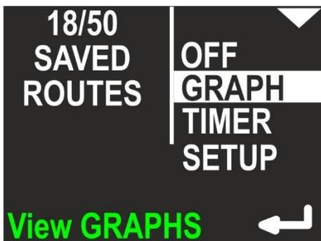
This function allows you to view the recorded data in the form of graphs on the screen of the device. A detailed description of the charts is provided in next chapters. After selecting this function, the left side of the screen shows the content of the memory - successively the number of already saved charts and the total memory capacity.
