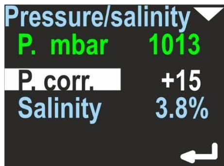
This option is used to control the work of the pressure sensor and to set the salinity necessary for correct (accurate) depth determination.
