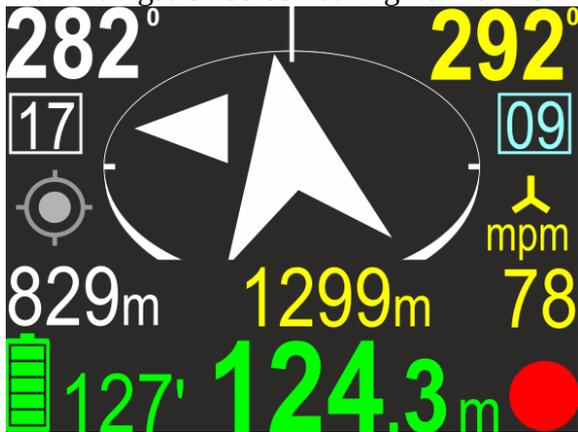
Main navigation screen if distance to the target is <20 m
