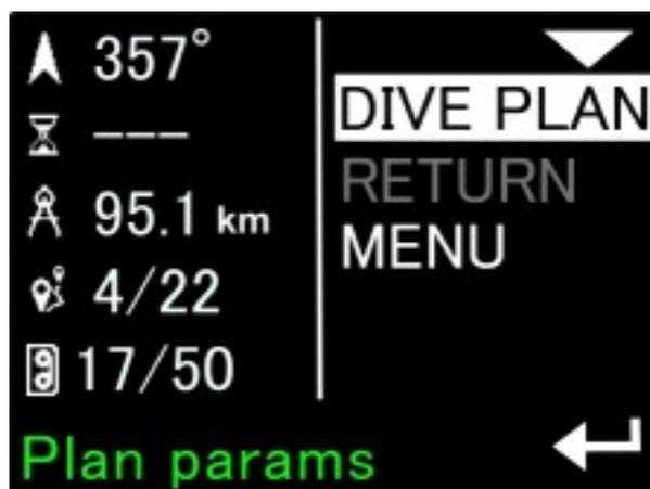
The right half of the screen will always contain three items. The first is information about the currently active navigation mode. It can be DIVE PLAN or Az./Dist. , as shown in the table above. Pressing the lower button of the console (SET) when the white frame with the check mark is set on this element leads us to the screen that allows you to program target settings, which will be described later in this study.
