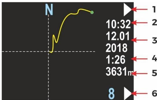
This screen presents the changes in the diver location projected on a flat surface (like on a map). The route start point is always positioned in the screen center. The route end point will be shown as a green dot, but only on the present route. Near the right edge of the screen, you will find some information elements:
