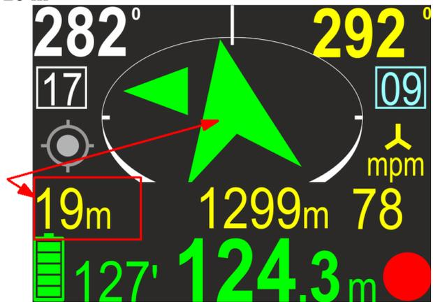
When the currently selected point is 10 meters or less - a text description (hint) associated with that point appears just below the compass arrow. This description is shown in blue for 3 seconds, alternating with the distance values (in yellow) that would normally be there.
