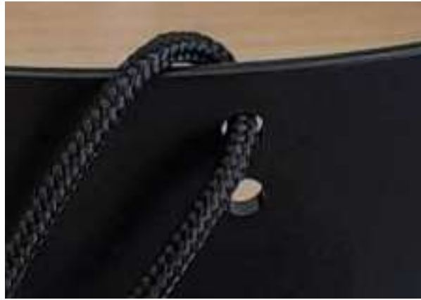
Fig. 11. Correct placement of the harness in the nozzle hole
