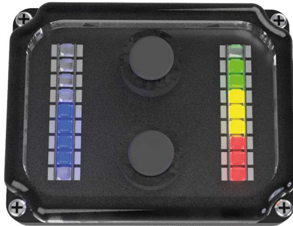
Fig. 21. Scooter switched on, gear 4 selected
