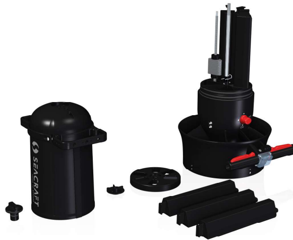
Fig. 25. Opened scooter with removed battery segments
