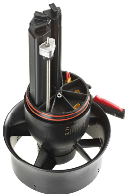
Fig. 27. Opened scooter with partly installed battery segments
