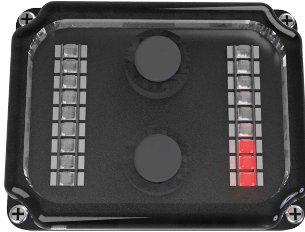
Fig. 23. Dropped battery capacity
