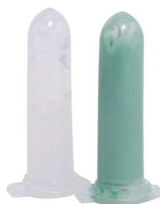
Fig. 15. Seacraft silicone grease and engine grease (green)
