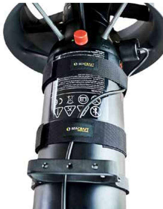
Adapter cable secured to the scooter (used for Seacraft SL52 light system)
